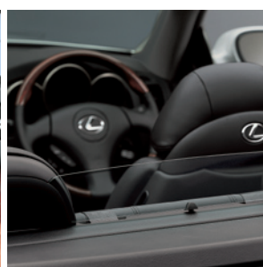
A WIND DEFLECTOR MINIMISES SWIRLING AIRFLOW.
